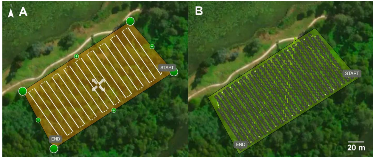
Figure 2.2. Flight path over the Yarramundi Reserve flying-fox roost: (A) shows the planned drone flight path; (B) shows the post-flight path, indicating where images were captured (black symbols; Pix4D, 2017) (background image source: Maxar).
