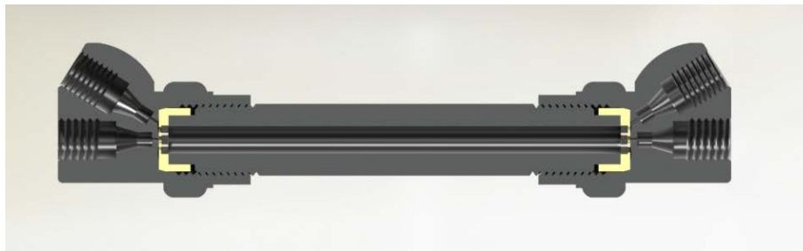
Figure 1.7 Curtain flow column with AFT fittings at the column inlet and outlet demonstrating the multi-port radial flow splitting process.
